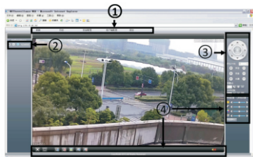
①主菜单 ②码流选择菜单 ③云台控制菜单 ④快捷菜单
